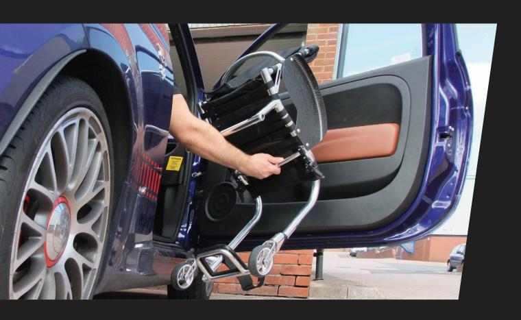
The made to measure frame includes the aluminum hand built frame which is designed to your individual requirements and the footrest, excluding the plate. Each tube has been reviewed and analyzed to ensure any excess weight is removed and the reliability is maintained.
