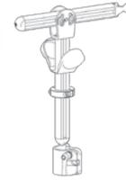
4. Attach base plate assembly and/or pads.
