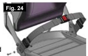
The lap belt is fitted to the wheelchair as shown in the illustrations. The seat belt comprises 2 halves. They are fitted using the existing seat stay retaining bolt fitted through the eyelet on the belt. The belt is routed under the rear of the side panel. (Fig. 24)
