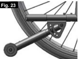
You must swing the anti-tips upwards when going up and down large obstacles (such as a kerb) to prevent them from touching the ground. Then rotate the safety wheels back down to the normal position (Fig.23).
