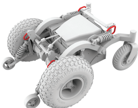
Figure 5.2c Frontier V4 lifting points
