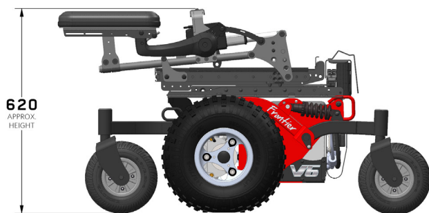
Figure 4.3c Frontier V6 and V4 Fold Forward height
