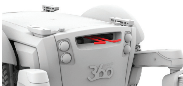
Figure 4.4b Magic 360 brake levers released
