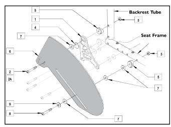
Figure D - Fixed Back, 1/4-in Offset
