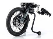
// STE060025 Mechanical double disc brake
