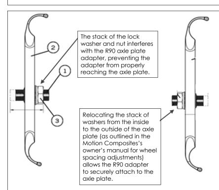
Section 8.11.5 of the Motion Composite Folding Wheelchair User Manual provides direction on how to move the washer and nut stack from the inside to the outside of the axle plate.
