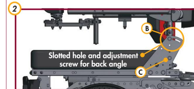
**ADJUSTING THE CENTER OF GRAVITY (Fig.3)**
