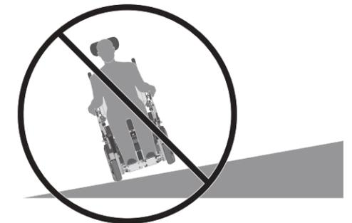
Figure 4. Do not turn on a slope.
