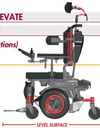
Tilt and Seat Elevate options are programmed to operate separately. The ability to tilt while the seat elevator is elevated is not possible. Bypassing this programming may cause severe injury.
