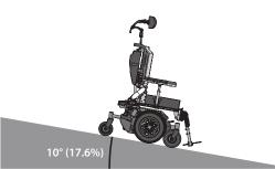
**Figure 3.** Do not use power wheelchair on slope steeper than 10°.
