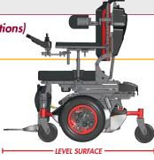
Tilt and Seat Elevate options are programmed to operate separately. The ability to tilt while the seat elevator is elevated is not possible. Bypassing this programming may cause severe injury.
