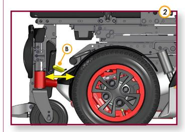
NOTE - For the freewheel position, if levers are difficult to engage or disengage, rock the wheelchair back and forth and/or push against the wheelchair while moving the lever.
