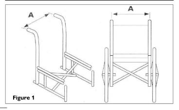
Next check that the back canes are a compatible diameter. The strap style back mounting hardware may be used on back canes from 0.62 to I. I inches (I 6mm to 28mm) in diameter. (Fig. 2)
